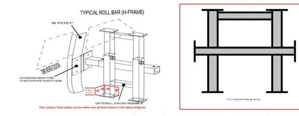
These two diagrams are a guideline to how the frame should be constructed but gusseting or triangulation is accepted.
